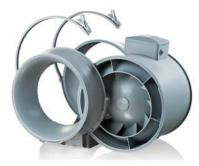
the spigots by means of special clamps with latches. This makes the fan maintenance fast and easy. The fan maintenance does not require total disassembling. Just pull out the central block from the casing and perform required servicing. All the models may be equipped with a regulated timer with turn-off delay adjustable from 2 to 30 min.
